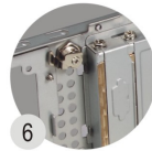
6 Kensington lock hole support and optional latch kits on back panel
