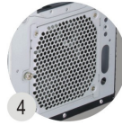
12cm fan and removable fan holder in the front and 8/9/12cm fan in the backplane (option)
