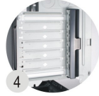
4 Screwless add-on-card devices installation (option)
