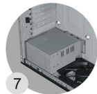
7 Power supply and a 12 cm fan install at bottom (option)
