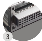
3 One-side-screwed mounted for 3.5" device
