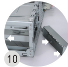
10 Support 2.5" HDD/SSD installation position 1
